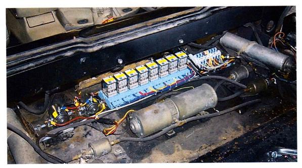
the above photo is of a typical installation in a 1964-66 Thunderbird. The relay system is of a previous design but the concept is the same. Do not follow the colors of the wires in this photo as it will differ from what you are about to do.
